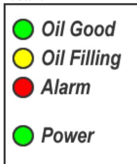
Oil Good (green colour): steady on while oil level is good, blinking for a first period of oil missing (even due to turbulence, undulations, etc.) before start filling and is off when filling.
