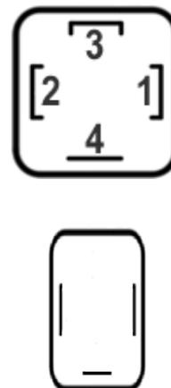
*The coil is connected between pins 1 and 2 and in the supplied harness is properly wired to the Electronic Module.*
