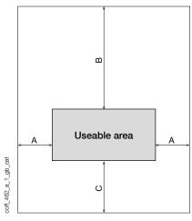
The useable area can be drilled for gland installation.
