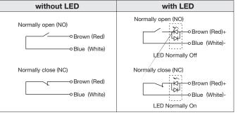
When using the switches with LED option, limit the current below 10mA.
