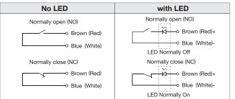
Electrical specification / circuit diagram. (Refer to P2-1) CL type interface unit cannot be used with LED.
