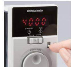
The motor's rotation direction can be switched with ease.
