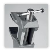
The SPANNFIX 9-205 is suitable for workbenches or work areas with a maximum table top thickness of up to 80 mm. The small vice with a ball joint can be attached quickly and easily to any workbench or worktop due to its table clamp. A small pressure of the lever is sufficient and the clamped workpiece can be fixed steplessly and in any practical working position.
