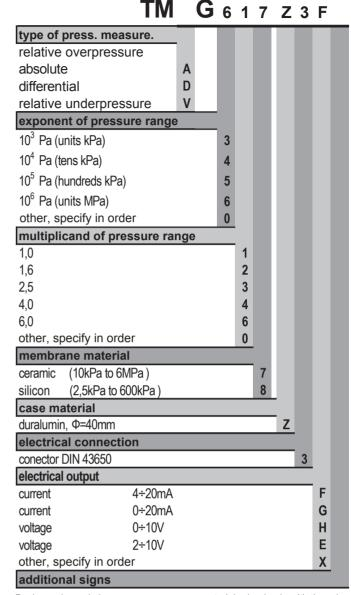
Basic version: relative overpressure, case material - duralumin with thread M12x1,5, conector according to DIN 43650, output 4÷20mA.
