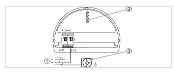
Electronics and terminal compartment, single chamber housing
