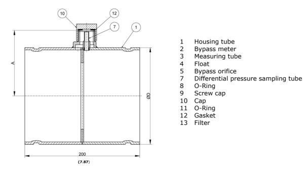
Fig. 7 FO Turbo-Lux 3 orifice plate, Drawing and dimensions 6"/ DN 150 - 8"/ DN 200 in mm (inch)
