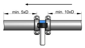
Fig. 1 Inlet path and outflow zone
