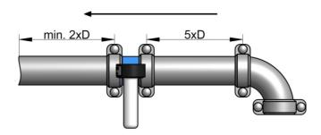
$\textit{Fig. 2} \ \, \text{Shortened inlet path and outflow zone}$
