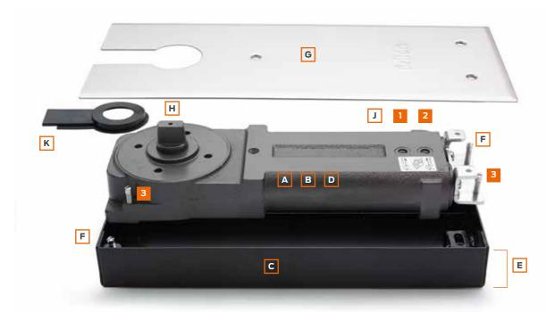
Adjustments: 1 - Closing speed (from 130° opening); 2 - Latch action; 3 - Lateral & vertical adjustment of the closer
