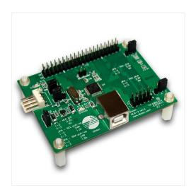
USB-I2C, USB-SPI, USB-GPIO interfaces, eight 10-bit analog inputs, 2 PWM outputs and two 32-bit pulse counters. Pulse counters, digital and analog inputs can send events to your application (e.g. when voltage level reaches the predefined value).
