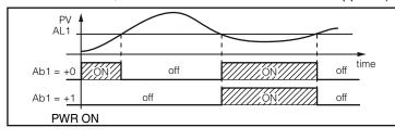
A "Latched alarm" (manual reset) is an alarm that remains active even if the conditions that generated the alarm no longer persist. Alarm reset can be done only by an external command ((u) button, digital inputs or serial link).
