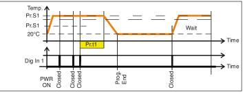
When a new panel is detected before the end of the first soak time, the program restarts and the set point remains equal to Pr.S1.
