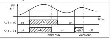
**4.** A "Relative alarm not active at set point change" is an alarm that masks the alarm condition <u>after</u> <u>a set point change</u> until process variable reaches the alarm threshold plus or minus hysteresis.
