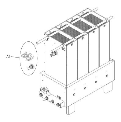
Figure 4. MICRODYN BIO-CEL® 104 exploded drawing of available accessories
