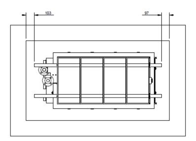
Figure 6. MICRODYN BIO-CEL\* 104 with accessories in standard filtration tank with minimum clearances (top and side view)
