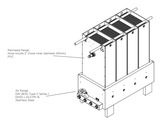
Figure 1. MICRODYN BIO-CEL® 104 scope of supply
