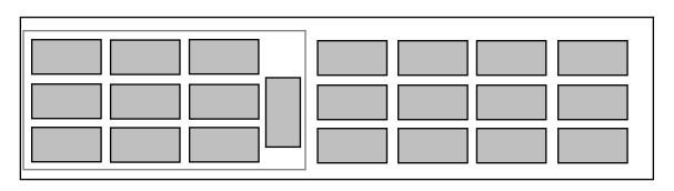
Figure 3. MICRODYN BIO-CEL\* 104 arrangement in 20/40 ft container (10 / 21 pcs capacity)
