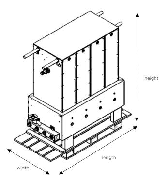
Figure 2. MICRODYN BIO-CEL® 104 in transport packaging
