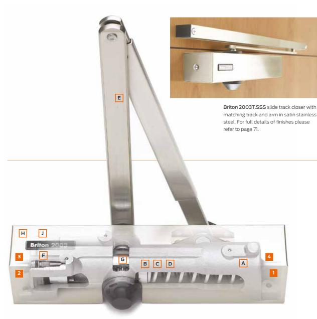
Adjustments: 1 - Closing power; 2 - Closing speed; 3 - Latch action; 4 - Backcheck
