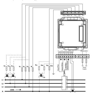
Direct phase-phase measurement with current transformers
