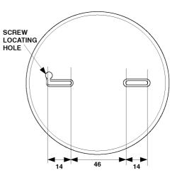
Fig. 1 Fixing Dimensions for Detector Base
