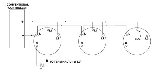
Fig. 6 Simplified Schematic Wiring Diagram
