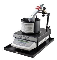
OHMIC Instruments Models UPM-DT-1PA & 10PA are precision wattmeters designed to measure the power output of diagnostic and therapeutic ultrasound transducers. The UPM-DT series have been in use worldwide since 1986 and conform to the testing guidelines recommended by FDA, JCAHO, AAMI and AIUM. Power is measured by the radiation methodand the accuracy of the UPM-DT's are traceable to NIST.
