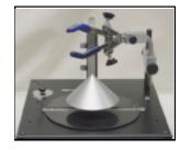
The cone target and transducer positioner. (Tank not shown.)
