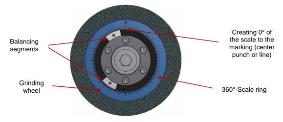
If no flange with balancing segments available, please ask for MPM balancing rings.
