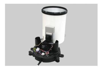
RG13H uses a pulse-based tipping-bucket mechanism to produce a contact closure every time it receives a predetermined small quantity of rainfall (0.1 mm / 0.004 in).
