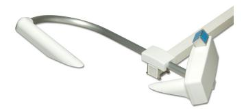
PWD12 and PWD22 identify precipitation type by accurately estimating the water content of precipitation with a capacitive device (Vaisala RAINCAP® sensor element) and combining this information with optical forward scatter and temperature measurements. These three independent measurements are processed through sophisticated algorithms in order to produce an accurate evaluation of the weather type according to the WMO and NWS code tables.
