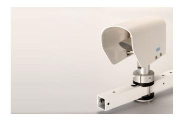
DST111 provides a unique remote alternative to measuring road surface temperature. By measuring the infrared radiation emitted by the surface and applying intelligent signal processing, the sensor provides a reliable remote surface temperature measurement.
