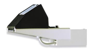
The DRD11A sensor offers fast and accurate precipitation detection and estimation about the intensity in the scale of low-mid-high. DRD11A has an in-built heating element for keeping the detection plate always ready for precipitation identification. The sensor requires periodical cleaning but is otherwise maintenance-free.
