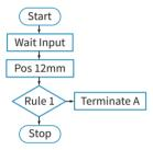
Entire motion sequences with up to 255 individual motion commands can be stored in the Command Table. This is primarily advantageous if complete motion sequences need to be executed very quickly, without dead time from the overlaid drive. In the Command Table, the programmer has access to all motion commands, internal parameters, and digital inputs and outputs.
