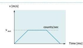
Synchronization to a belt speed can be done using the Master Encoder Interface or Step/Direction/Zero interface. Applications such as the "flying saw", synchronous loading or unloading, synchronous filling or labeling of bottles or containers on a conveyor belt, and many other applications can be implemented in this way.
