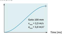
For direct position targets, using absolute or relative positioning, the desired position is reached using acceleration and velocity-limited motion profiles or jerk optimized profiles (jerk limited and Bestehorn). Positioning commands can be invoked via the serial interfaces, CANopen, DeviceNet, Profibus, Ethernet or a trigger input.
