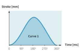
For synchronization to an external main or master shaft, the linear motor travels along the motion profiles stored in the drive, at the machine speed (machine angle 0...360°). Using this function, mechanical cam discs can be replaced with highly dynamic linear motors. The motion profiles can be freely defined, and the correct motion profile can be invoked during product changeover with no changeover time.
