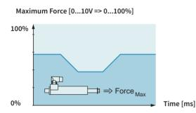
Easy Steps provide the ability to parameterize internal parameters using two analog inputs. If, for example, the maximum motor current is read at an analog input, then the maximum motor force can be provided as analog for freely programmable joining processes.
