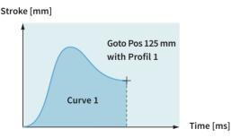
For travel to an absolute position, or shifting by a relative position, any desired motion rules can be stored besides the VA interpolator. They are stored in the drive as motion profiles (Excel CSV format). The positions can be approached, for example, with a sinusoidal motion to optimize power loss, or special reverse optimized motion profiles.
