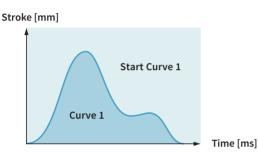
Up to 100 different time curves can be stored Series E1200 drives, with up to 16,000 individual waypoints. The motor can thus travel along time curves of any complexity, such as those generated by CAD programs and stored in the drive (Excel CSV format). The time curves can be invoked via the serial interface, fieldbusses, ETHERNET, or the trigger input.
