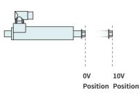
For an analog position target, the linear motor travels to a position proportional to the input voltage. The position is either scanned continuously, or only after a rising edge of the trigger signal. In order to prevent uncontrolled jumps in position, the motor travels to the positions with a programmable maximum acceleration and velocity (VA interpolator).
