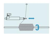
For winding textile yarns, glass fiber optics, or wires, a complete functional block is available that controls the entire sequence of a complete winding process.
