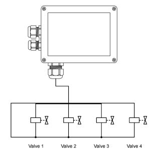
solenoid valves integrated into the casing
