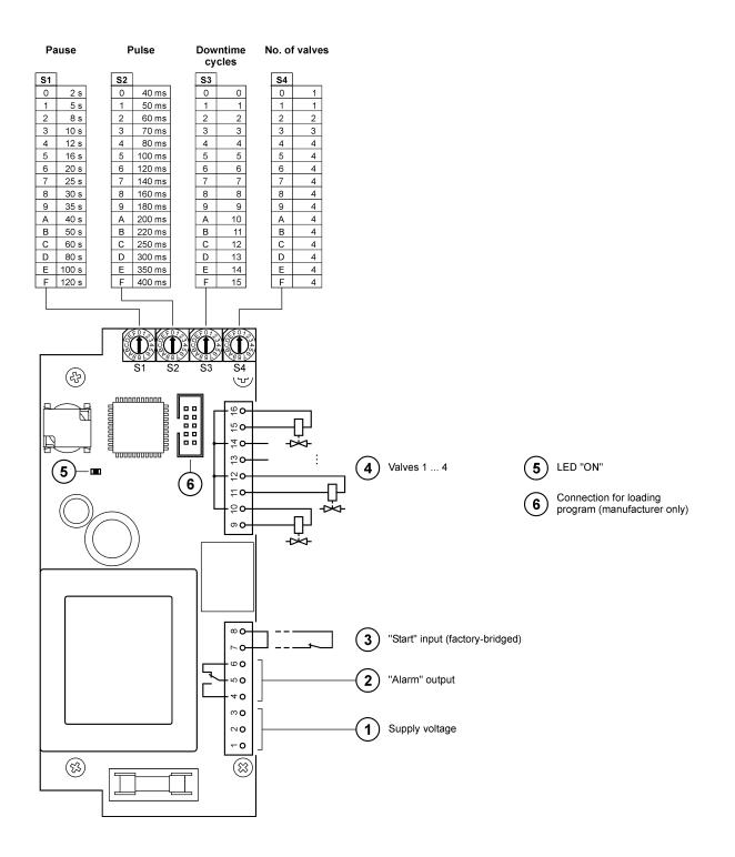
Figure 3: Layout of the RM-BV 4 Micro circuit board and connection plan
