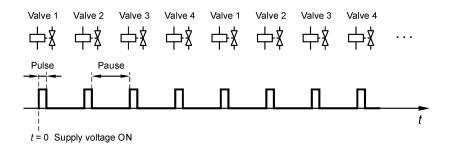
Figure 1: Standard operation of filter control system RM-BV 4 Micro
