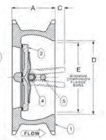
**NOTE:** Twin Disc Check Valves can be installed horizontally or in the vertical position with flow up.
