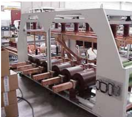
> AGN-24 Transformer for generator switchgear.
