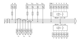
Connection of 3 phases + neutral 1 current transformer
