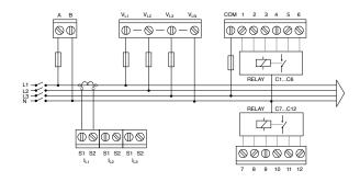
Connection of 2 phases + 1 current transformer
