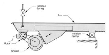
In this design, the drive location is chosen so that the force generated by the Shaker is directed through (or near) the system's center of gravity. The motor terminal box must be packed with insulating putty to prevent vibration of the wires; connect utilizing flexible cable.
