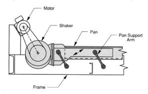
This design is used when full access to the pan is required, but is impractical to mount the drive below the pan. Shaker may be mounted with feet perpendicular to the pan as shown, or with feet parallel to pan arms. In either case, the V-belt centerline must be parallel to pan arm supports.
