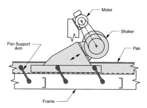
The shaker drive can be located anywhere along the pan, but usually inward from either end. Motor is attached to an extension of the stationary base frame. Note that shaker feet and V-belt centerline are both parallel to the pan support arms.
