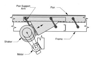
Use of this design allows full access to the conveyor pan.
