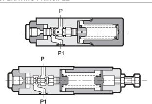
The MZD valve is a three-way spool type direct operated pressure reducing valve. It is normally open in the rest position and the hydraulic fluid passes freely from the P1 line to the P line.
