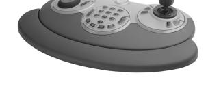
The **KBD5000** Series keyboard is the controller for Pelco's complete network-based video system products. It is the point from which all user functions can be accessed. The KBD5000 Series is compatible with all Endura® Series distributed, network-based video products.
