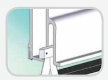
The top of the blade is captured within the extrusion, ensuring that a perpendicular cut is achieved.
