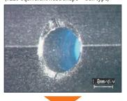
The edge shape is broken & secondary burrs are generated **Edge quality: Poor**
