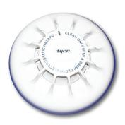
The MR601TEX overcomes the slower response of optical detectors to hot burning fires by increasing the sensitivity of the optical detector when it is associated with a rapid change in temperature. In this way it is intended to become a detector which will suit some of the risks currently covered by ion chamber detectors. Smoke detectors will not detect burning alcohol or other clean burning liquids which do not generate smoke particles.
