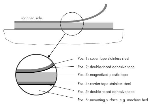
Figure 1 Components of the Magnetic Tape
