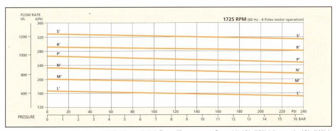
Characteristics at constant motor speed, with water at 68 °F and by-pass blocked - Figures of flow are averages - Pump weight: 1,9 kg (4,2 Lbs) clamp mount and 2 kg (4,4 Lbs) flange mount
