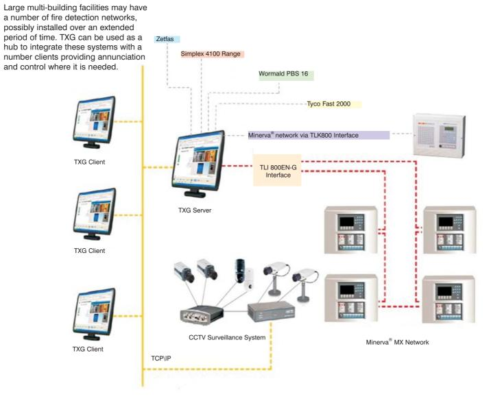
TXG with multiple fire detection networks and CCTV integration
