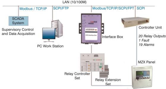
By means of the Relay Controller Set and the Relay Extension Set an additional 256 relays per sensor cable can be connected.
