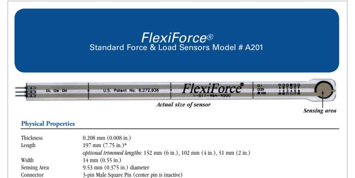
Substrate Polyester (ex: Mylar) Pin Spacing 2.54 mm (0.1 in.) \* Length does not include pins, please add 31.75 mm (0.25 in.) for pin length to equal a total length of 203.2 mm (8 in.).
