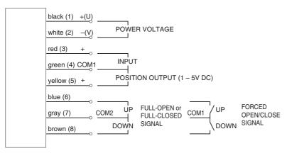
■ With Both Full-open/closed Signal and Forced Open/Close Signal
