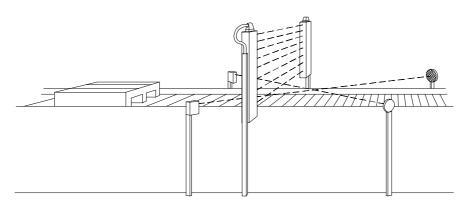
Figure 13 Assemble the barrier with the connectors to the top.
