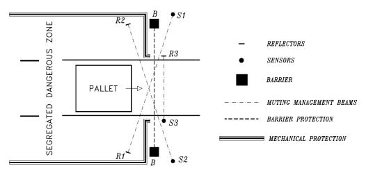
Figure 4 Positioning of sensor 3 in a typical application.
