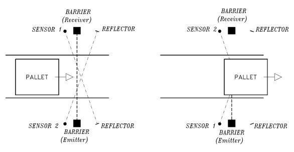
Figure 1 Positioning of the safety barrier and of the muting sensors.
