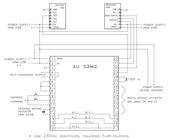
\*\* When wiring between OVdc and  $\pm$  is foreseen, jumper the control unit terminals 2 and 3.
