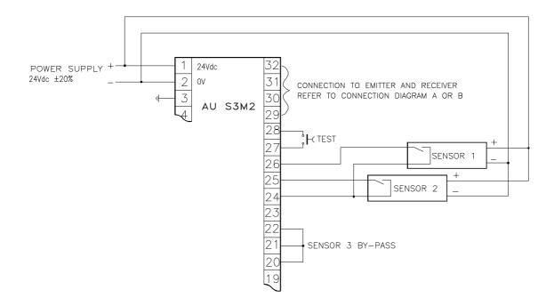
Connection to muting sensors with PNP static output: use of sensor 3.
