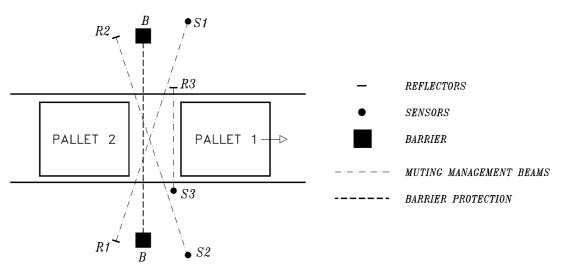
Figure 3 Sensor 3 and pallet separation.
