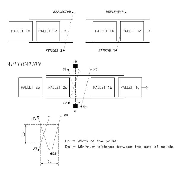
Figure 11 How to keep sensor 3 occupied with very close pallets.
