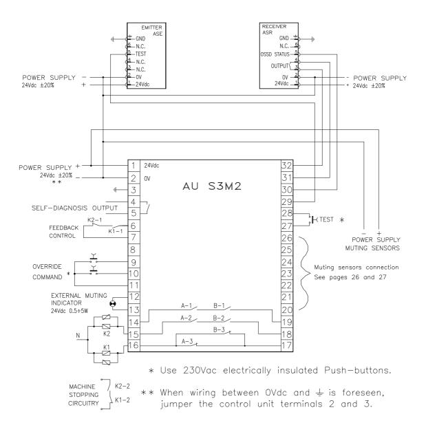
Connection to muting sensors with relay output: use of sensor 3.
