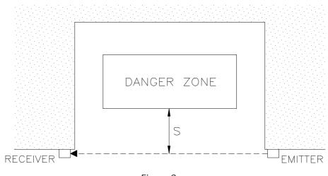
Figure 8 Comply with the minimum safety distance.
