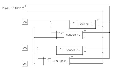
Figure 14 Parallel connection of proximity type muting sensors.
