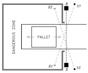
Figure 12 Entry/exit type bi-directional system: sensor 3 cannot be used.
