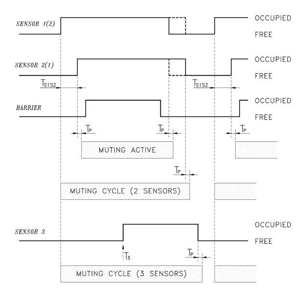
Note: The signals represent the voltage logical levels at the inputs of the control unit.
