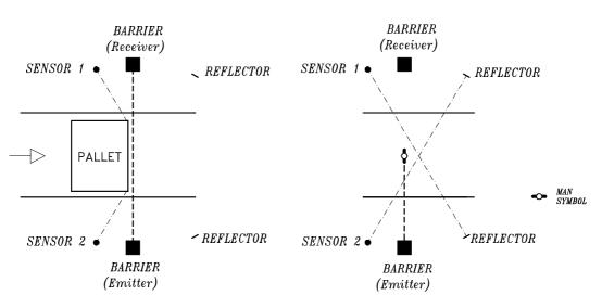
Figure 2 Positioning of the muting sensors.
