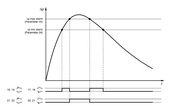
The setting  $\Delta p$  min alarm switch point (Parameter 04) = 0 deactivates the differential pressure monitoring function  $\Delta p$  min alarm.
