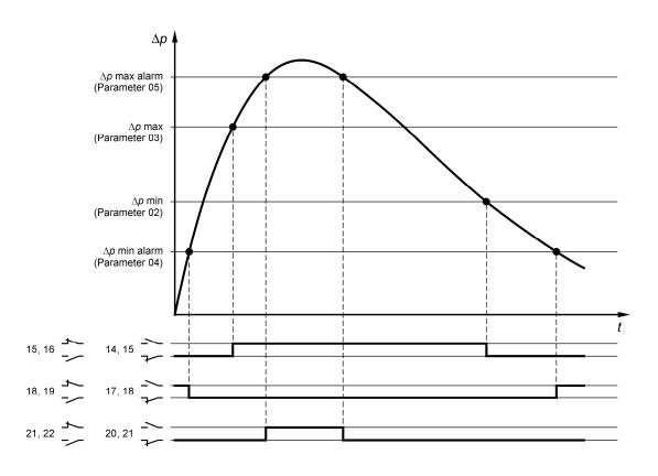
The setting  $\Delta p$  min alarm switch point (Parameter 04) = 0 deactivates the differential pressure monitoring function  $\Delta p$  min alarm.
