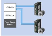
When using PLC, an operation system can be configured by connecting directly to an I/O module. A positioning module is not necessary on the PLC side, so space is saved and the system is
