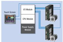
Normally, the motor is started and stopped with I/O. Changing the operating data settings and displaying the monitors and alarms are performed with the touch screen using Modbus (RTU) communication. When there is a lot of setup work, changes can be easily made on the touch screen, which reduces the burden of
