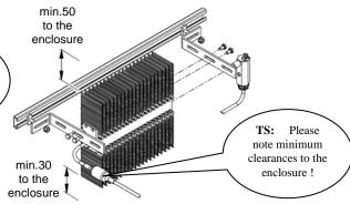
The brackets in zinc coated steel and fixing bolts illustrated above are included with the heater.
